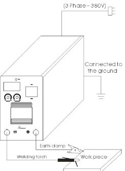
According to input voltage grade, connect power cable with power supply box of relevant voltage grade. Make sure no mistake is made and make sure the voltage difference is among permission range. After the above job, installation is finished and welding is available.
